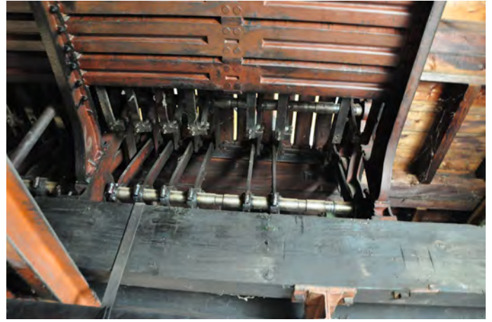
2024, underside of lever frame located in locking room (ground floor). Source: Heritage Victoria
