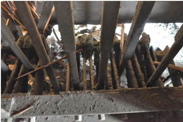
2024, rods and pulleys at base of lever frame located in locking room. Source: Heritage Victoria
