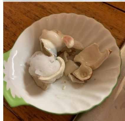
Example of a damaged object: increased humidity caused the salt to expand and crack a rabbit salt shaker.
