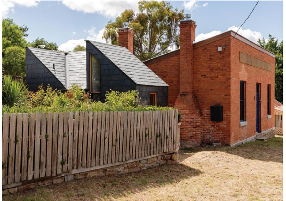
The extension to the Bank at Vaughan is clearly contemporary. The form of the 'pod' is inspired by the steep skillion roof of the bank building. Clad in a different but equally robust material (slate), it is connected to the original by a glazed link, which provides a clear visual separation between old and new.
