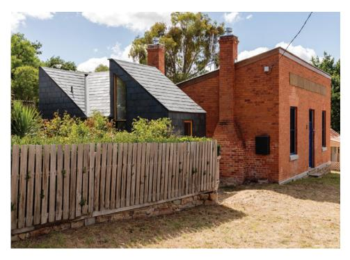
The extension to the Bank at Vaughan is clearly contemporary. The form of the 'pod' is inspired by the steep skillion roof of the bank building. Clad in a different but equally robust material (slate), it is connected to the original by a glazed link, which provides a clear visual separation between old and new. **ARCHITECT:** MARIA DANOS ARCHITECTURE. **PHOTOGRAPH:** TREVOR MEIN.
