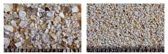
**Figure 19: Grading of sands.** The sand on the left is well graded. It has a wide range of particle sizes from very coarse through coarse, medium, fine and very fine. The sand on the right is poorly graded, with a relatively uniform (fine to medium) particle size. Each division on the scales in these photographs is 1 mm; each image is about 20 mm across.
