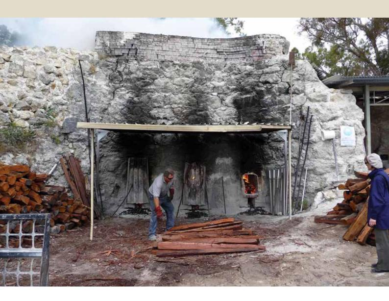
Figure 7: Traditional lime burning. A lime kiln at Susac Lime Supply, Carabooda, north of Perth, Western Australia. This may be the last such lime kiln operating in Australia: most had ceased production by World War II.
