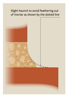
**Figure 70: Avoiding feathered edges.** To avoid feathering, finish the tail of a joint with a slight haunch, which can be shaped by tamping with a bundle of bristles.
