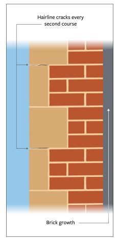
**Figure 73: Brick growth.** In this sectional view of a composite wall, brick growth has lifted the stones, producing a hairline crack at every second bed joint.
