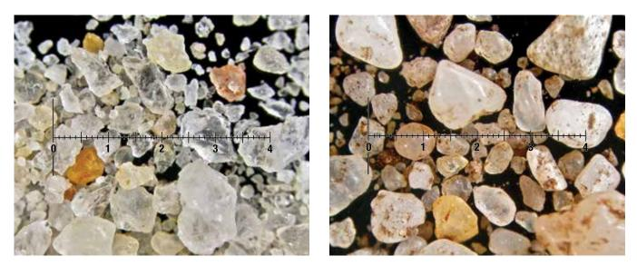
**Figure 18: Surface texture of sand grains.** The sand on the left has angular to sub-angular (sharp) grains, while that on the right has rounded to well-rounded grains. Sharp sands make strong mortars; rounded sands don't. Another aspect of these sands is that the one on the left has been washed clean, while the one on the right has clay coatings on the grains, which will weaken a mortar made from it (see Section 9.5). Scale bars in millimetres; each small division is 0.1 mm (100 µm).
