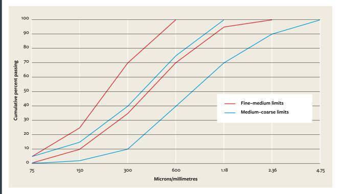
**Figure 22: Proposed size-grading envelopes.** Cumulative plots of proposed envelopes for fine-medium and medium-coarse sands. The plot for a particular sand should ideally lie approximately parallel to the envelope boundaries. A medium-grained sand suitable for 5–7 mm joints should plot close to the overlap between the two envelopes shown here. Sands may need to be screened to reduce the maximum particle sizes to suit particular joint widths.
