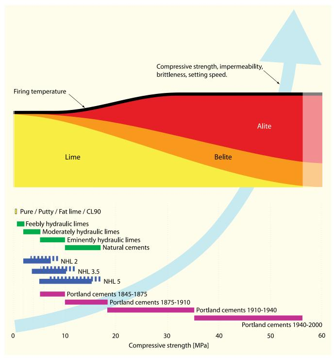
**Figure 14: The lime-cement spectrum.** The diagram shows the continuous range of materials from pure (non-hydraulic) lime on the left through the hydraulic limes to modern cements on the right. Their increasing strength and other properties are shown against firing temperatures and the changes in their lime and silicate chemistry. The diagram simplifies complex data and boundaries are approximate only.
